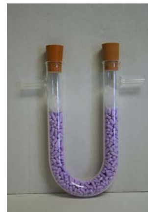
Fig. 6. 15g AMSORB PLUS desiccated by oxygen
